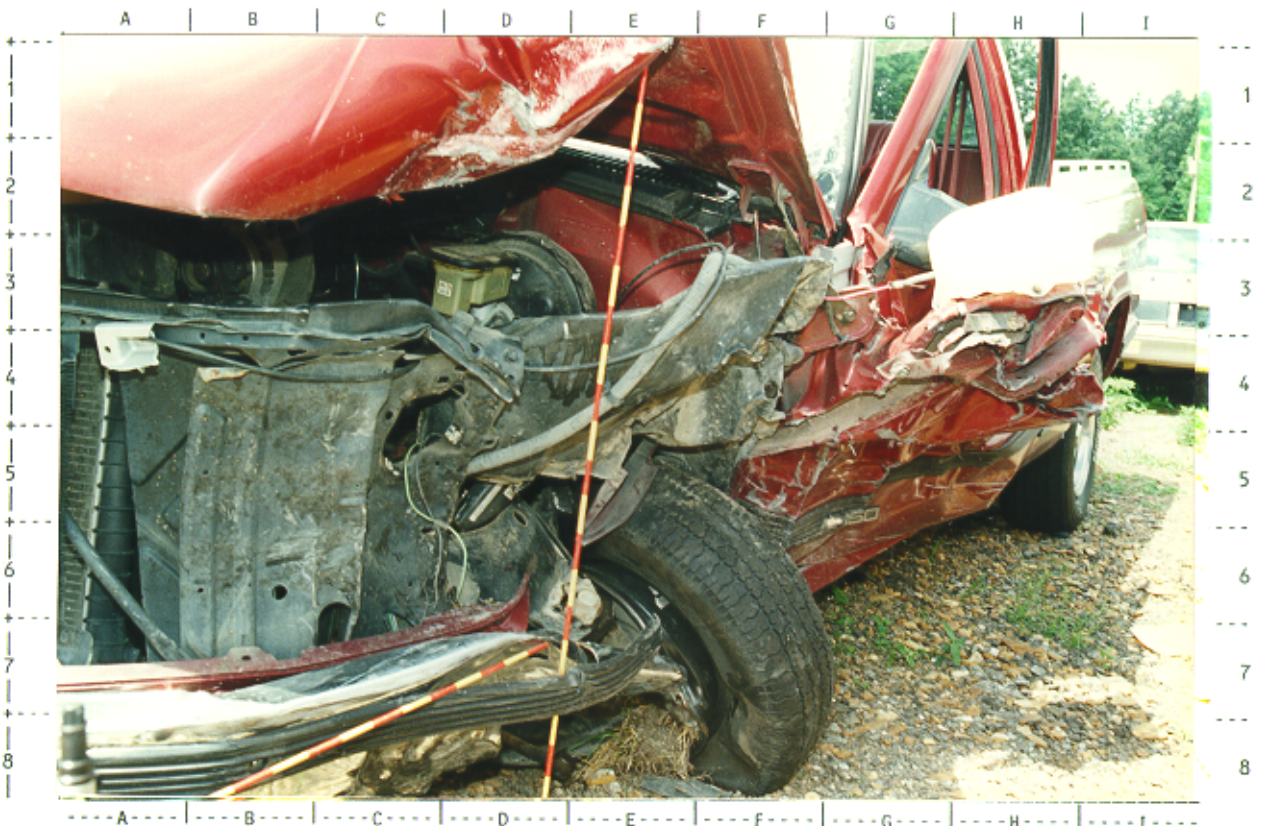
# 66 -- Front left close-up of damage to 1988 Chevrolet pickup; NOTE: damage to FL hood, LF wheel, & continuation along left side
